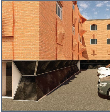
Figure 16: Protruding brick façade creating high contrasting shadows to deter rats. Source: (Image by Author 2024)
