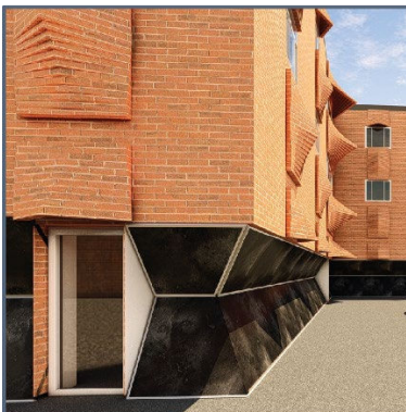
Figure 18: Angled metal panel at the ground plane to deter rats. Source: (Image by Author 2024)
