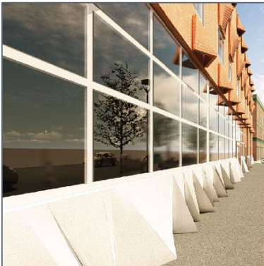
Figure 17: Dimensional concrete facade at the ground plane to deter rats. Source: (Image by Author 2024)
