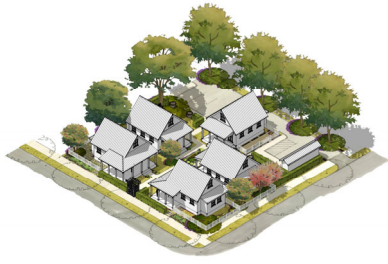
Figure 2.6: Axonometric drawing showing the layout of a Bungalow court: (Congress for the New Urbanism)
