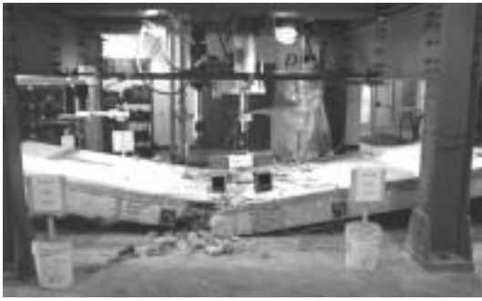
Fig. 18—Flexural failure of Bridge Model BBD-I.
