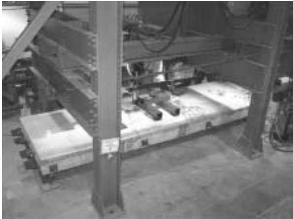
Fig. 13—Test setup for box-beam Bridge Model BBD-I.
