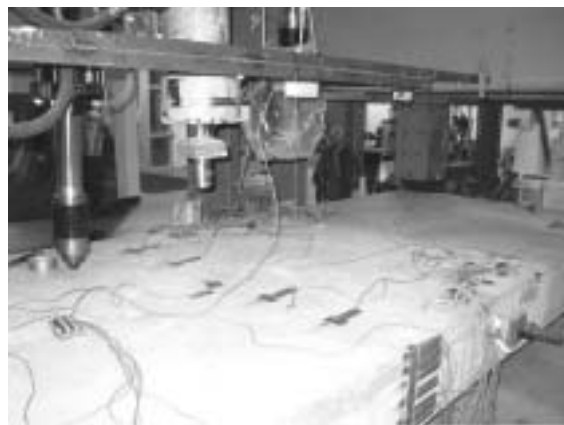
Fig. 12—Arrangement of linear motion transducers and strain gauges before testing of Bridge Model BBD-I.
