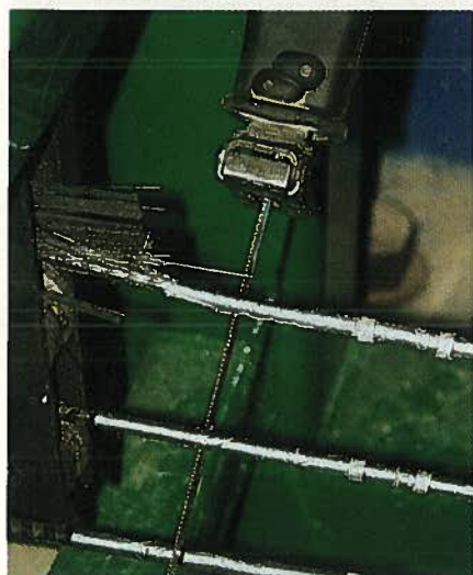
Fig. 10. Sudden release of Leadline™ prestressing tendons using hand-held saw.
