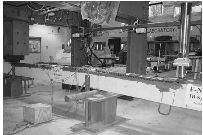
Fig. 10—Failure of Beam F-NV.
