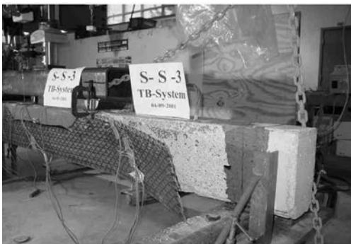
(c) Failure of beam S-S-3
