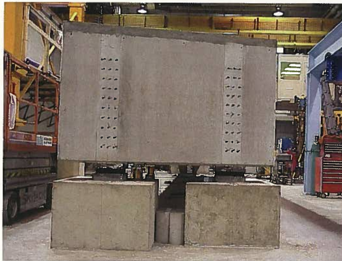
Fig. 10. Flexural load testing at the CTL testing facility.
