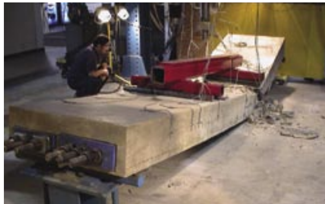
Fig. 3: Shear failure of box beam M2 with S A stirrups
