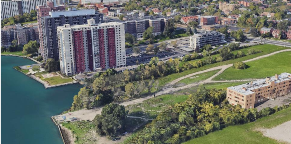
Figure 18: An aerial view of two waterfront residential towers shows how much surface parking is required for such buildings. The surface parking footprint is almost three times that of the building. Though surface parking is convenient and offers an organized way of parking, it leads to greater amounts of contaminated runoff making its way into the river.
