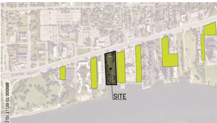
Figure 18: Retrofitting the vast impervious footprint within the immediate context of the site will yield multiple green spaces, reduce impervious surfaces, and subsequently reduce urban runoff.
