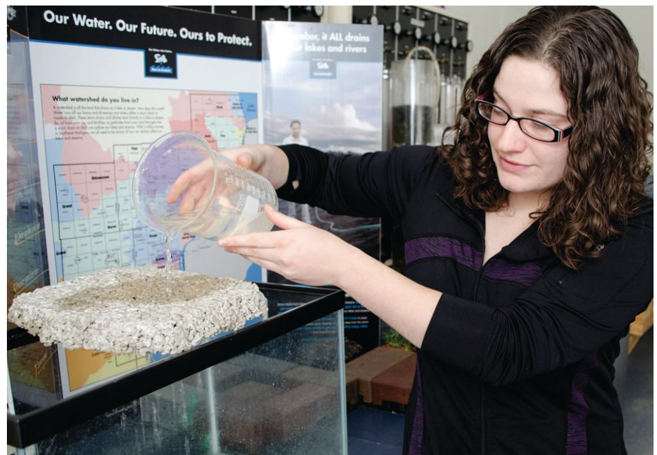
LTU civil engineering graduate student Rachel Pieschek demonstrates how porous paving materials reduce stormwater runoff by letting water flow through.
