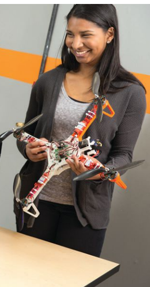
Robotics engineering students Mark Kenney and Kristin Jordan hold polylactic acid plastic parts for a quad copter that were printed on one of the Makerbot 3D printers in LTU’s Prototype Lab.
